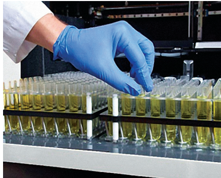
Intelligent racks make it possible to automatically manage the location of sample tubes.
